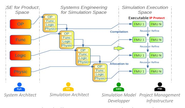
FMI standard allows to preserve the know-how of the stakeholders in an Extended Enterprise How do we ensure the consistency of simulation models?
